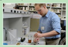
John Wulterkens (Technical Service Engineer) showed his group how to troubleshoot VpCI®-377 application problems with a refractometer. Measuring product solution concentration with a refractometer can help the distributor decide if the customer needs a higher concentration of the fluid to prevent rust, or if contamination (indicated by a falsely high concentration reading on the refractometer) is causing product performance problems.
