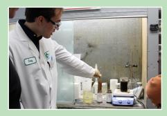
Casey Heurung (Technical Service Engineer) demonstrated rust removal and the benefits of heating VpCI®-422 to speed up the process. He also showed how unheated VpCI®-422 removes rust much more slowly, and how VpCI®-426 is a quicker rust removal alternative in situations where it would be difficult to heat VpCI®-422.
